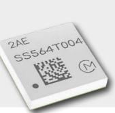
The Murata Type 2EA is a Wi-Fi 6E plus Bluetooth BR/EDR/LE 5.3 module based on the new Infineon CYW55573 Chip with tri-band capability (2.4GHz, 5GHz and 6GHz) and 2×2 MIMO. It has a small form-factor of only 12.5 x 9.4 x 1.2 mm and connectors for external antennas. It can be used in applications in the Smart Home area like e.g. camera systems, as well as in AV/VR applications.
