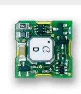
Ultra-low power DC/DC converter for thermal energy harvesters.
